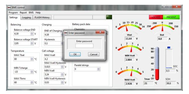
Once you unlock the BMS, you get a permission to change the original settings on the device. The sign in the right top corner should change to UNLOCKED.
