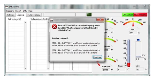
The BMS is not connected to the BMS Control software, the sign NOT PRESENT is turned on and Reading BMS configuration window pops out. Click the "Cancel" button and open Set communication properties in the Program menu.
