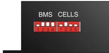
**Figure 3:** BMS address and cell selection DIP Switches.
