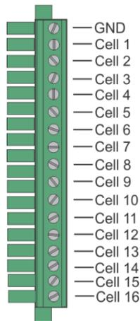
Figure 6: Battery pack to BMS connection.
