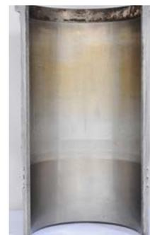
Even after 7,000 hours of operation, the liner above shows that the exceptional anti-wear and dispersant technology in Mobil Pegasus 605 Ultra 40 prevented scuffing, bore polishing and the formation of lacquer.
