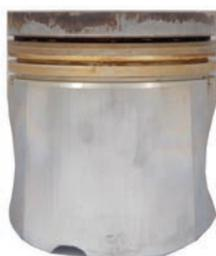
After 11,899 operating hours on Mobil Pegasus™ 605 Ultra 40 (35,519 total engine hours), critical components were removed and evaluated. Power cylinder assemblies showed minimal carbon deposits, varnish and lacquer in piston lands and grooves.
