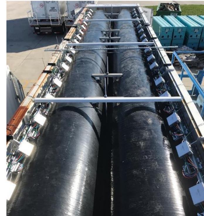
*In-situ MAE Requalification of TITAN@ and SMARTSTORE@ Modules/Cylinders*
