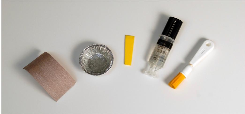
These tools are needed to repair Level 2 damage (left to right): 120-grit (fine) sandpaper, a receptacle for mixing epoxy resin, a resin applicator, two-part epoxy resin (resin plus cure) and a brush that may be needed for removing dust and debris. Clean shop rags or heavy-duty paper towels are also useful.
