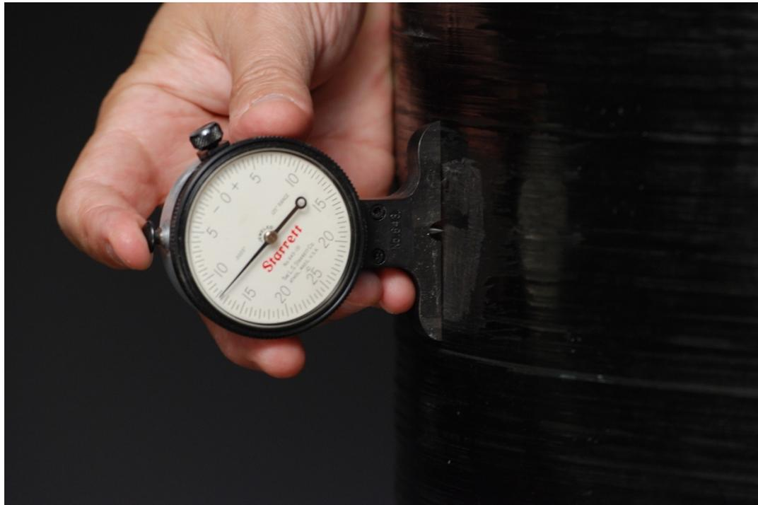
▲ **Abrasion measurement**—Calibrate the depth gauge to zero on the undamaged cylinder surface (left), then measure the depth of the abrasion at the deepest point (right).
