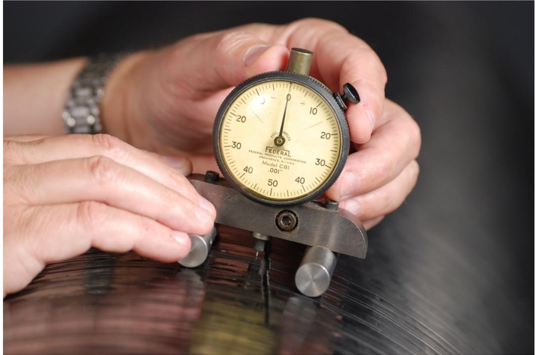
▲ **Cut measurement**—First calibrate the depth gauge to zero on the undamaged cylinder surface.
