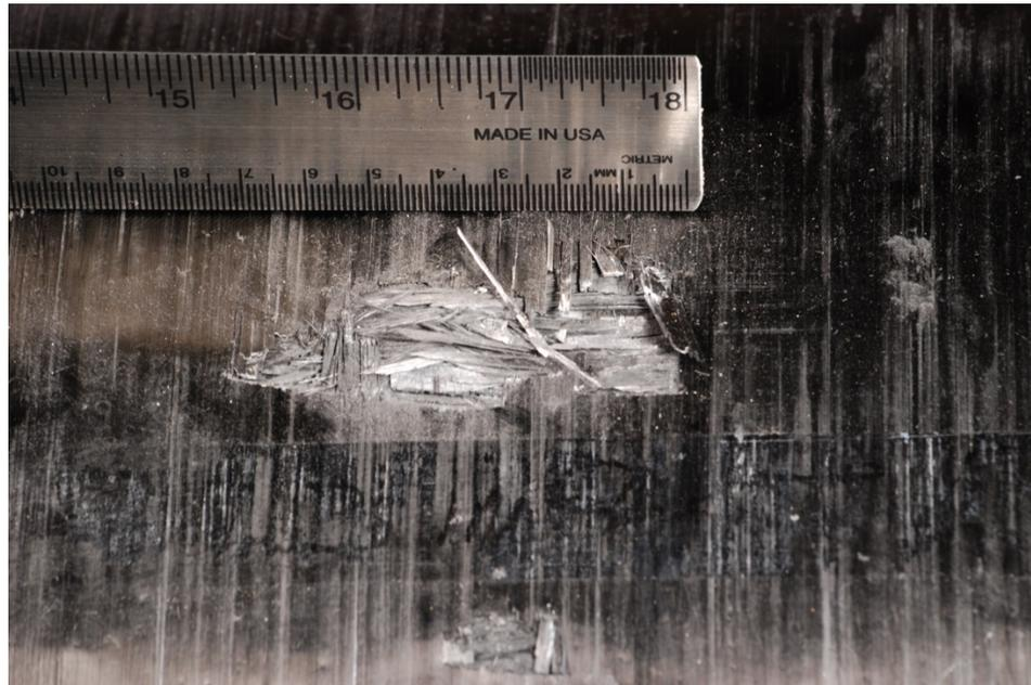
▲ **LEVEL 3:** Severe damage in which impact has caused a large area of frosting (including cuts or abrasion), damage to fibers in the cylinder dome, liner denting
