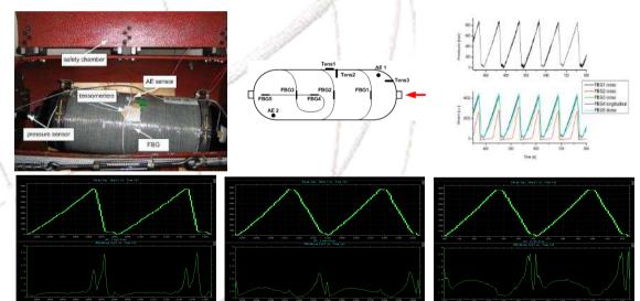
Pressure (upper graphs) and RMS signal from acoustic emission sensors (bottom graphs) at different moments of the experiment
