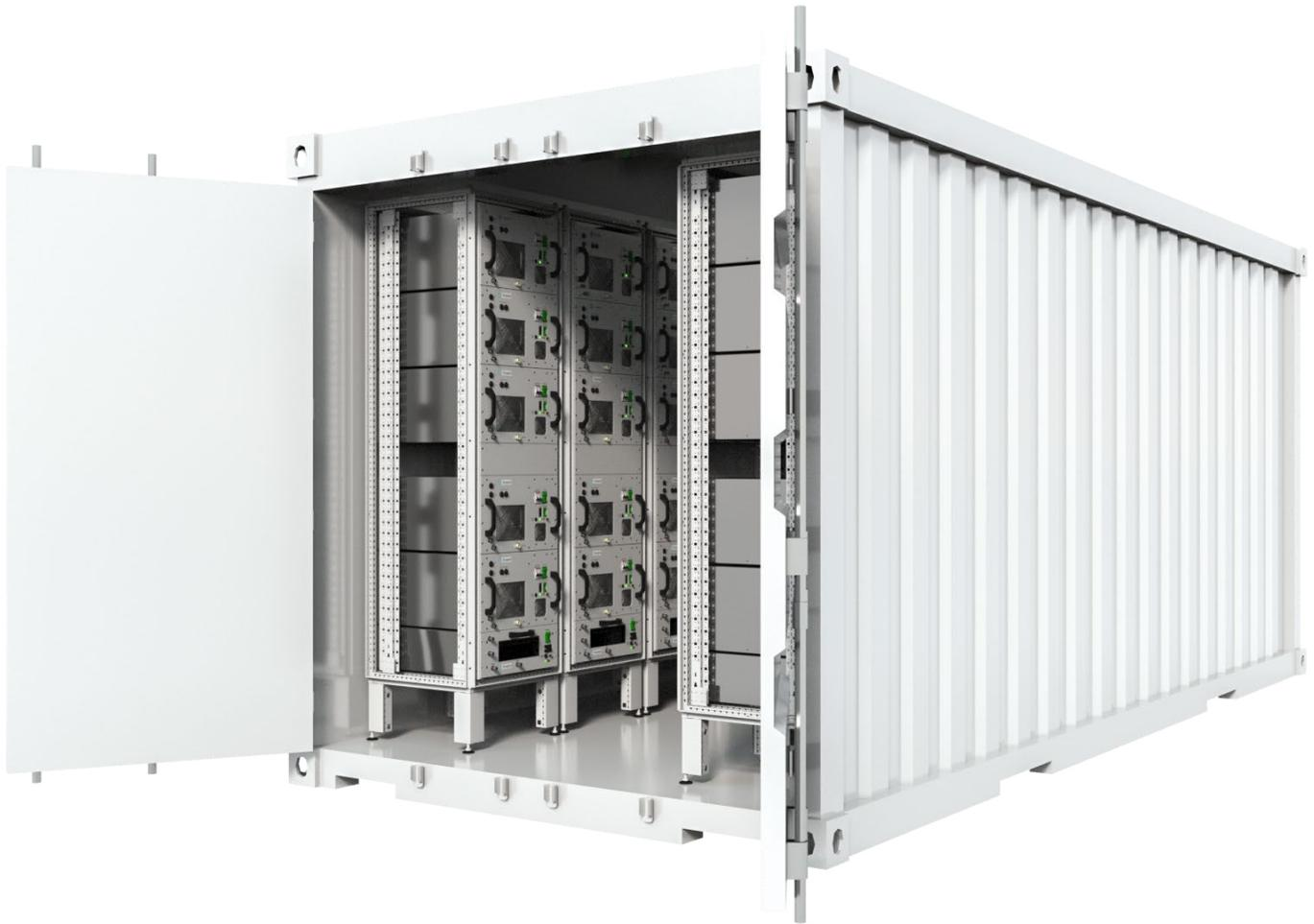
The Enapter AEM Cluster 60 is a fully assembled, ready to run and packaged electrolyser system in a 20' container. It supplies hydrogen with a rate of 30Nm<sup>3</sup>/hr at 99.999% purity. Site works are limited to the connection of vent and purge lines, water supply, hydrogen outlet piping as well as grid connections.
