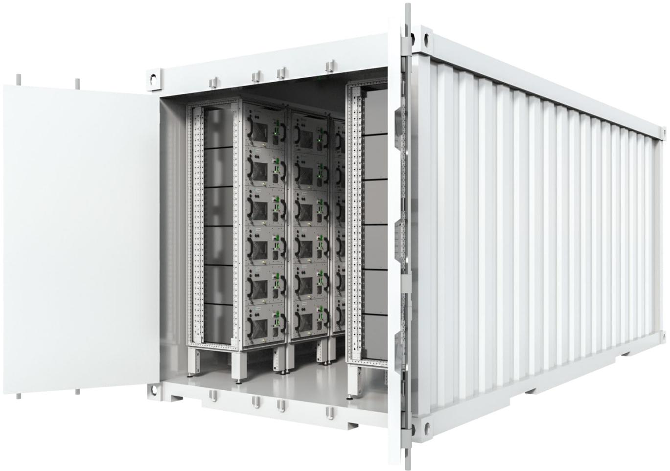
The Enapter AEM Cluster 70 is a fully assembled, ready to run and packaged electrolyser system in a 20' container. It supplies hydrogen with a rate of  $36\text{Nm}^3/\text{hr}$  at  $\sim 99.9\%$  purity. Site works are limited to the connection of vent and purge lines, water supply, hydrogen outlet piping as well as grid connections.
