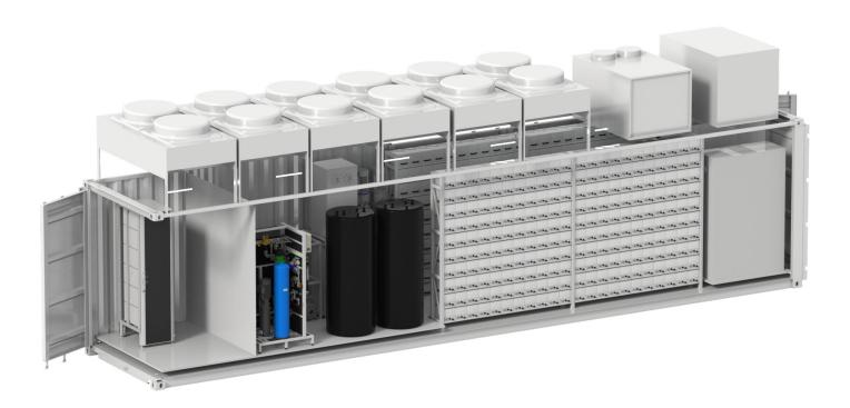
The Enapter Electrolyser AEM Multicore is fully assembled, ready to run and packaged in a 40' container. Site works are limited to the connection of vent and purge lines, water supply, hydrogen outlet piping as well as grid connections.
