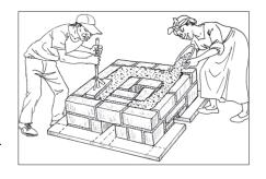
**4.1** Build up the second course of bricks for the outer wall, and mortar them into position.
