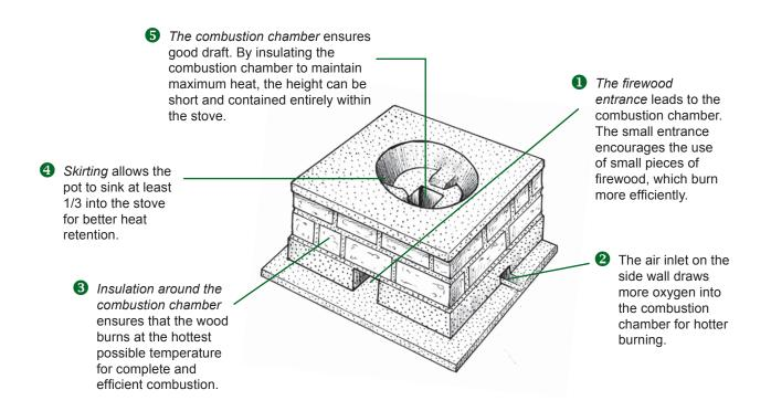
The combustion chamber of the rocket stove increases draft to enable almost complete burning, hence higher temperatures up to 600°C. This leads to faster cooking, with less firewood and less smoke.
