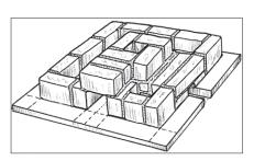
**3.2** Place the bricks for the outer wall of the stove, leaving space for insulation between the outer and inner walls. Mortar the bricks into position to complete the first course.
