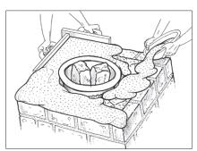
6.4 Pour mortar on the surface and spread out evenly. Smooth it to about 2.5cm from the edge of the pot. Ensure that the stove's top surface is uniformly horizontal.
