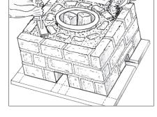
**6.3** Pour ash or gravel into the gaps between the pot and the outer wall. Compact the insulating material, then sprinkle with a little water as before to prepare the surface for mortaring.
