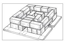
**4.2** Pour the clay mixture into the gaps between the combustion chamber and the outer wall, up to the level of the bricks. This is for insulation. Press down lightly to compact the material so little air remains.
