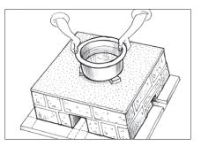
**5.1** Around the combustion chamber, place 3 pieces of cut brick to make the pot rests — 1 at the back wall, the other 2 on either corner of the front of the chamber. Add mortar as a base to hold the pot rests in position.
