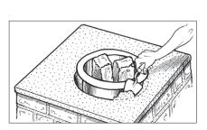
**7.3** Scoop out the excess mortar inside the line, going down to the level of the pot rests.
