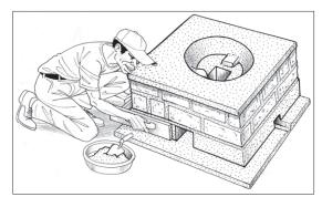
**7.5** Use the extra mortar to smoothen the sides and add finishing touches, such as the skirting around the stove.
