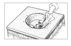
**7.4** Remove the pot and smoothen the sides of the pot rest area, using a little mortar. Wear a rubber glove or protect your hand with a plastic bag. Keep excess mortar for the finishing touches.
