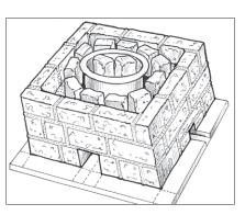
**6.2** Cut 4 or 5 bricks into half and stand the pieces in a circular pattern around the pot, making sure the pot is in the centre.
