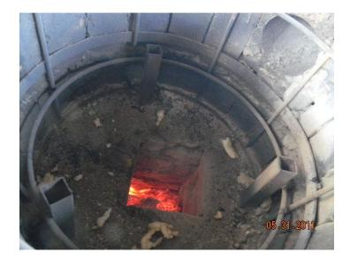
FIGURE 8 Concentrated heat improving the fuel efficiency of the New Stoves
