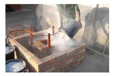
FIGURE 5 FILLING THE LOWER STOVE BODY WITH INSULATING MATERIAL (ASH). THE POT SUPPORT HAS BEEN LAID ON TOP OF THE GRATE
