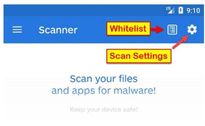
Before going any further, two settings at the top of the Scanner page should be mentioned. **Whitelist** is used to exclude some files from being scanned as part of a normal scan. **Scan Settings** allow you to define if scheduled scans are to be performed, when they are to be performed, and if scans should be run based on certain device events. **Whitelist** is covered on page 11 and **Scan Settings** are covered on page 13.
