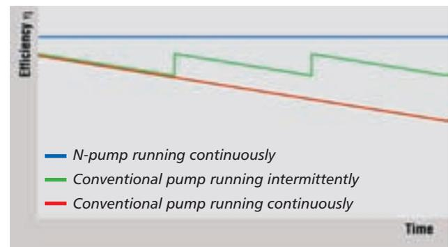
■ The red line shows how efficiency decreases when a conventional wastewater pump clogs during continuous operation.
