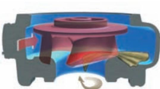
Stage two: rags get fed into the relief groove as the impeller turns, pulling them from the impeller and forcing them into the volute where they get pumped away.
