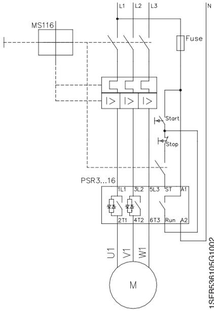
C) With fuses, contactor and O.L.
