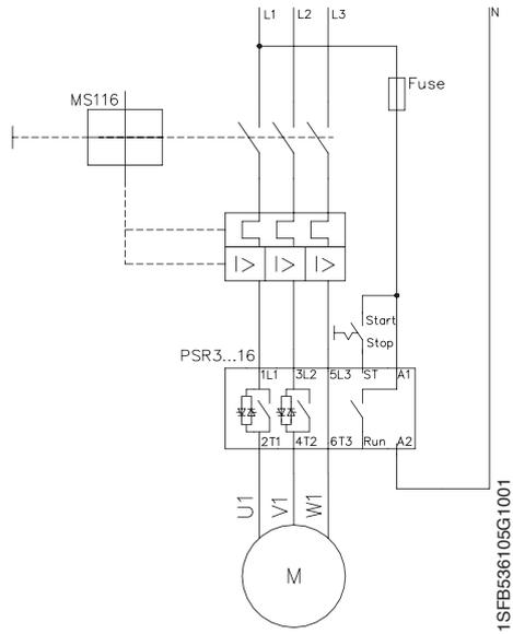
B) With MMS and auxiliary contact
