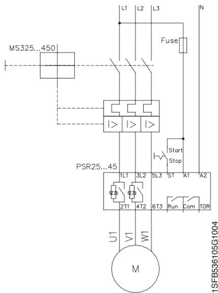
E) With MMS and auxiliary contact
