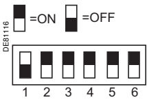
Converter positioned at end of bus
