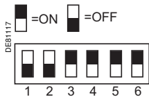
Converter not positioned at end of bus
