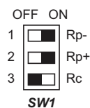
Converter not positioned at end of bus
