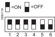
Converter positioned at end of bus
