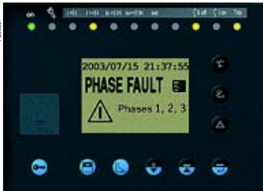
Local indications on the Sepam front panel.
