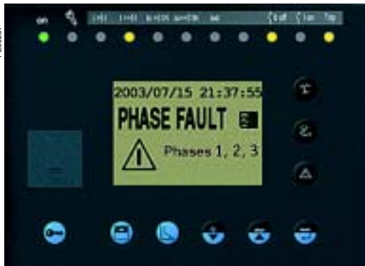
Local indications on the Sepam front panel.
