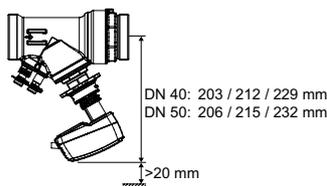
TA-Slider 750/1600 / TA-Slider 750/1600 Plus, Fail-Safe Plus
