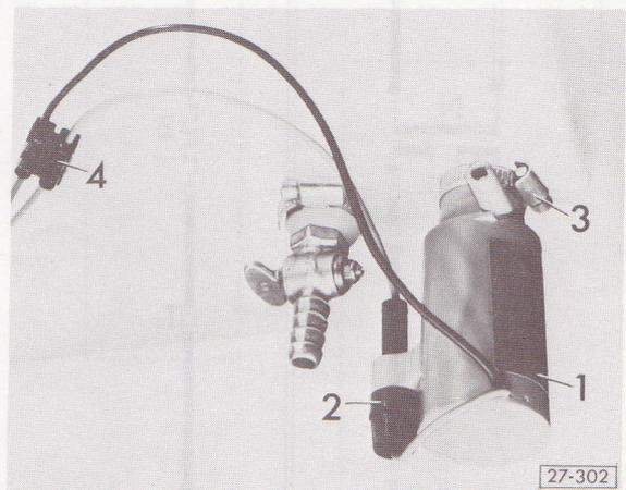
**Fig. 5** Sink water pump, removing/installing
